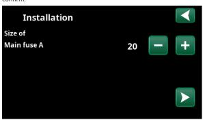
4. Select the size of the main fuse using the "+" and "-" buttons. Confirm with the "right" directional arrow. For more information about settings, refer to the "Installer/Settings/Immersion heater" chapter.
