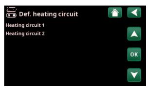
Menu: "Installer/Define/Heating Circuit". Select a heating circuit and press "OK" to access the settings.
