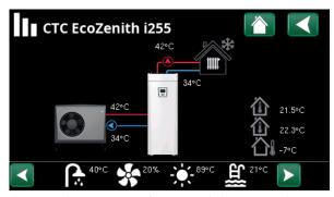
The screen shows operating information with the CTC EcoAir heat pump connected.
