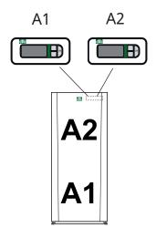
The left-hand display is connected to the bottom cooling module (A1) while the righthand display is connected to the top cooling module (A2). When more than one product (two cooling modules) is connected, the subsequent cooling modules must be addressed correctly. The CTC Basic Display on these products can be used to name these products as shown below, see the manual for the CTC Basic Display.
