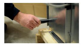
2. Attach the two carrying handles to the bottom of the cooling module.
