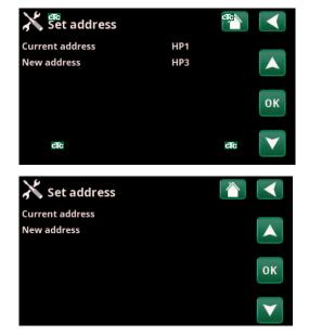
When all heat pumps are numbered and energised, they should be displayed when you press the heat pump symbol in the menu "Operation data". If any heat pump does not appear in the menu (communication with the heat pump fails) It may be because it has not been numbered as described above.
