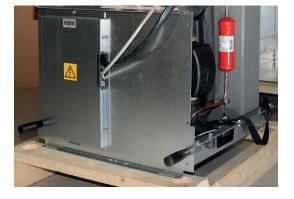
6. Lift the cooling module into the product using the carrying handles and shoulder straps. Remove the carrying handles and reconnect the power cable, hoses and screws. Installation and Maintenance Manual
