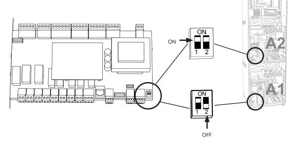
DIP switch 1 is used to set whether a CTC Basic Display is connected. This is why it is set to OFF on the Pro version and ON on the standard version of the heat pump.
