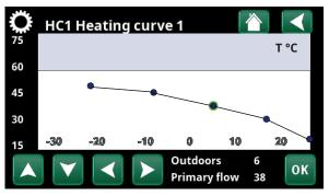
Menu: "Installer / Settings / Heating Circuit / Heating Circuit 1/Heating curve/Fine adjustment".
