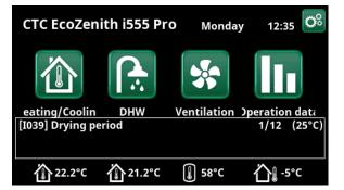
Example: Drying period temperature day 1 of 12 with current set point of 25 °C.
