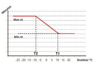
The diagram shows that the heating time of the heating coil to the condensation trays is regulated depending on the outside temperature.
