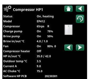
The menu shows detailed operation data of the selected heat pump. If the system includes several heat pumps, click the desired heat pump in the "Status heat pump" menu to access this menu.
