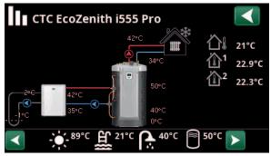
Main menu page for "Operation Data" with liquid-to-water heat pump CTC EcoPart connected.
