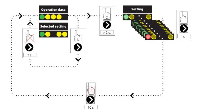
1. Briefly press the circulation pump arrow to show the operating mode to which the pump is set. After 2 seconds, the operational information screen will be displayed again.
