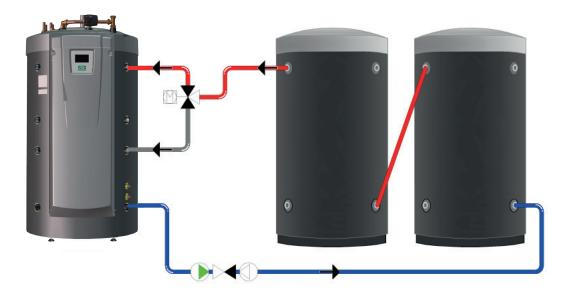
Recharging from buffer tank to the EcoZenith is always performed to the upper tank, if possible. If charging to the EcoZenith's upper tank is not possible due to too low a temperature difference, the controller checks if charging to the lower tank is possible. The condition for recharging is a 7 degree temperature difference.
