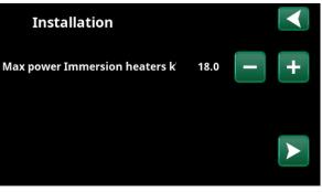
6. Select maximum immersion heater power using the "+" and "-" buttons. Confirm with the "right" directional arrow. For more information about settings, refer to the "Installer/Settings/Immersion heater" chapter.
