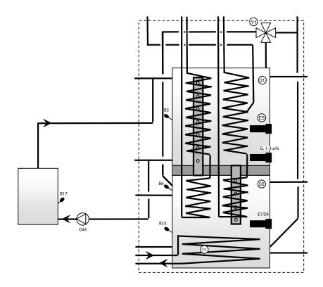
NB: Connecting with charge group reduces the potential risk of condensation forming and corrosion in the hearth.
