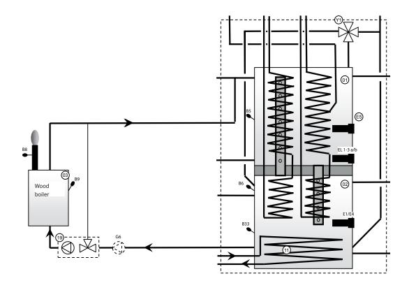
NB: Connecting with charge group (19) reduces the risk of condensation forming and corrosion in the hearth.
