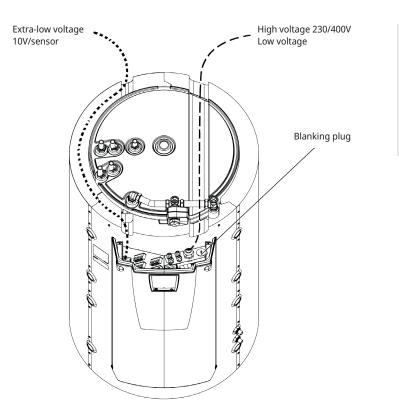
It is important to keep high voltage and extra-low voltage cables apart in order to avoid interference problems; this applies outside the product also.
