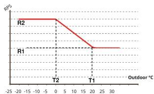
The diagram shows that the compressor speed is controlled according to the outside temperature.
