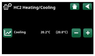
In the menu, "Cooling" (setpoint: 20.0 °C) is active for heating circuit 2. "Holiday mode" (V) does not lower the setpoint when cooling is active.
