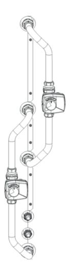
If ports ▲ and ■ have been shifted during the hydraulics connection, the motor can be reconnected to change its direction of rotation. This is done using two jumpers inside the motor. **NOTE! The direction of rotation cannot be changed by swapping the black and brown cables.**
