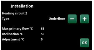
8. Specify whether heating circuit 1 applies to radiators or underfloor heating. Switch between "Radiator" and "Underfloor Heating" by clicking the (+) and (-) buttons. Confirm with the "right" directional arrow.
