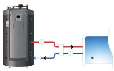
A pool is connected to the EcoZenith's lower tank. Between the EcoZenith and the pool, a heat exchanger is installed to separate the liquids.
