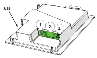
The back of the display unit has 3 communication ports.
