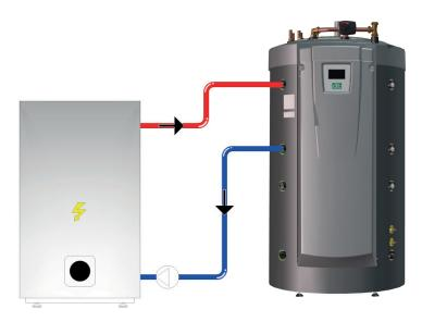
After a certain delay, which is factory set at 120 minutes, the unit with low priority is also started and helps the heat source with high priority.
